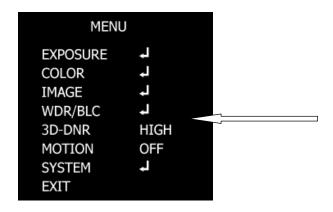
Switch to HIGH, MIDDLE, LOW and OFF to enable or disable noise reduction on dynamic recordings.
